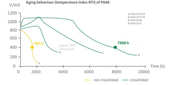
The test describes the aging behaviour of a plastic after storage at high temperature. PA66 not crosslinked only has 50% of its electrical insulation properties after about 800 hours. A crosslinked polyamide achieves a tenfold service life.
